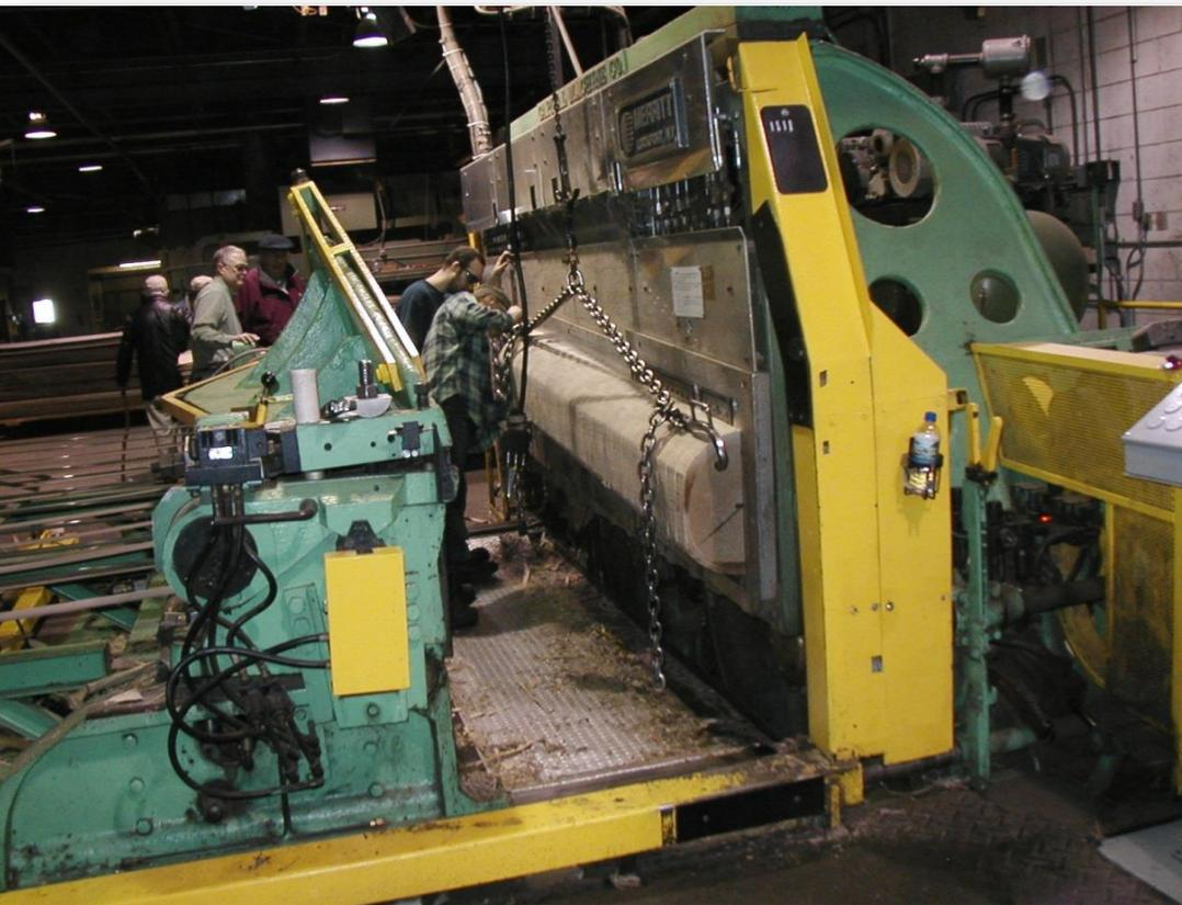
**Figure 3. Loading a half log onto a veneering machine**
